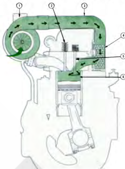
Fig. 5-16 Intake air flow schematic -KT(A)-19 engine
